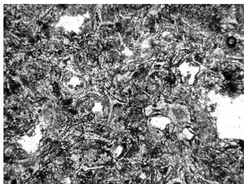
Fig. 2. Microphotographs of the zeolitized Oaxaca pyroclastic rocks showing perfectly preserved original shape of completely zeolitized glass shards (left) and zeolitized pumice clast with spherical bubbles (right). The light zones are zeolites, the dark ones are clays; plan-polarized light
