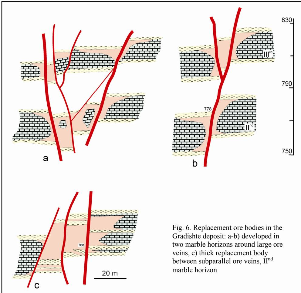
Fig. 6. Replacement ore bodies in the Gradishte deposit: a-b) developed in two marble horizons around large ore veins, c) thick replacement body between subparallel ore veins, II<sup>nd</sup> marble horizon
