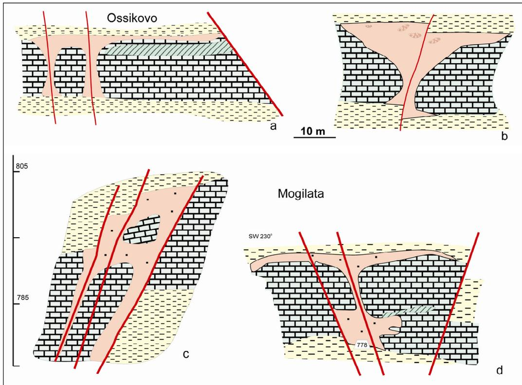
Fig. 7. Columnar, mushroom-like and irregular in shape replacement bodies in the Ossikovo (a) and Mogilata (b-d) deposits, developed around non-mineralized faults
