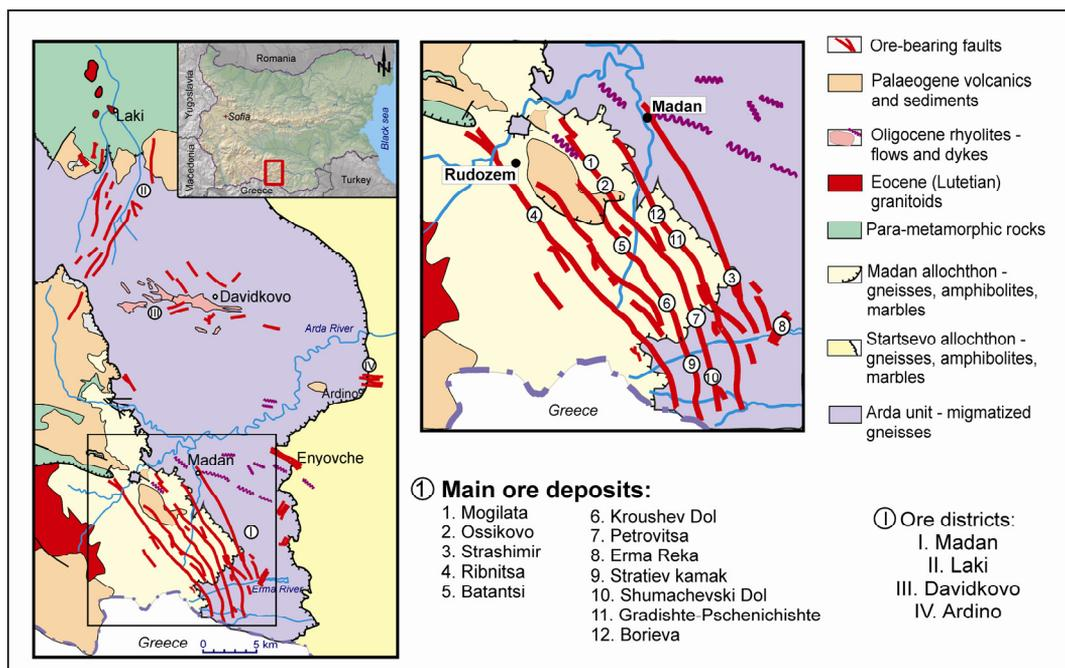
Fig. 1. Simplified geological map of the Central Rhodopean Dome and main ore districts attached to it in Bulgaria (modified after Ivanov 2000)
