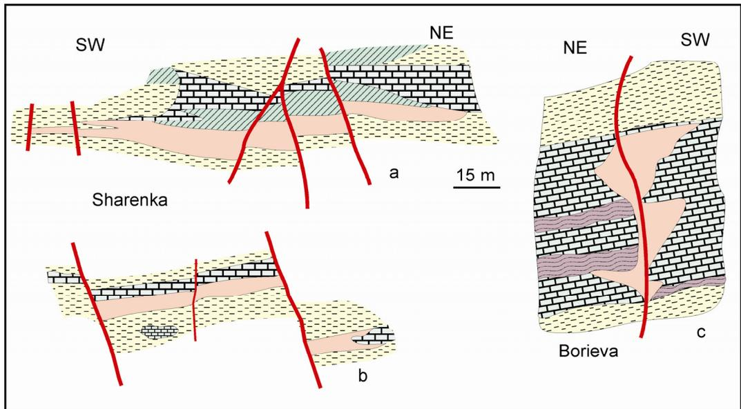
Fig. 8. Cross sections of metasomatic bodies in the III<sup>rd</sup> marble horizon from Sharenka (a, b) and Borieva (c) deposits (modified after Dokov et al. 1962)
