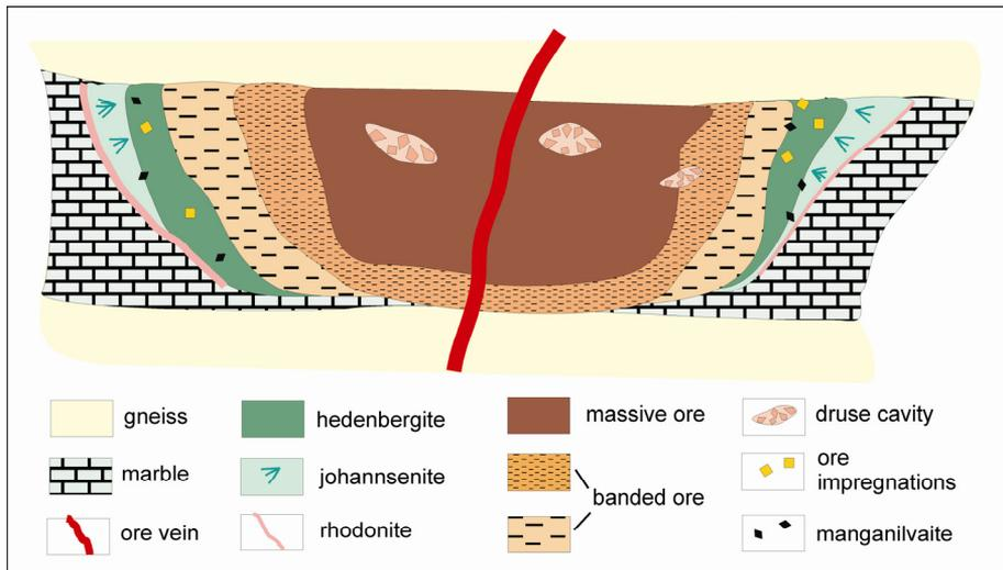
Fig. 4. General distribution of zones in a replacement ore body
