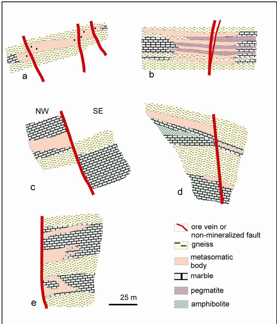
Fig. 5. Sections from several deposits in the Madan region: a) thin marble layers entirely mineralized, Pshenichishte deposit; b) skarn-ore ledges intercalated with pegmatites and gneisses, Nadejda; c) massive bed-like body in the footwall of a strongly denivelated marble layer, Enyovche; d) bed-like bodies around the ore vein, Kroushev Dol; e) irregularly-shaped metasomatic bodies at mining level 450 in the Kroushev Dol deposit
