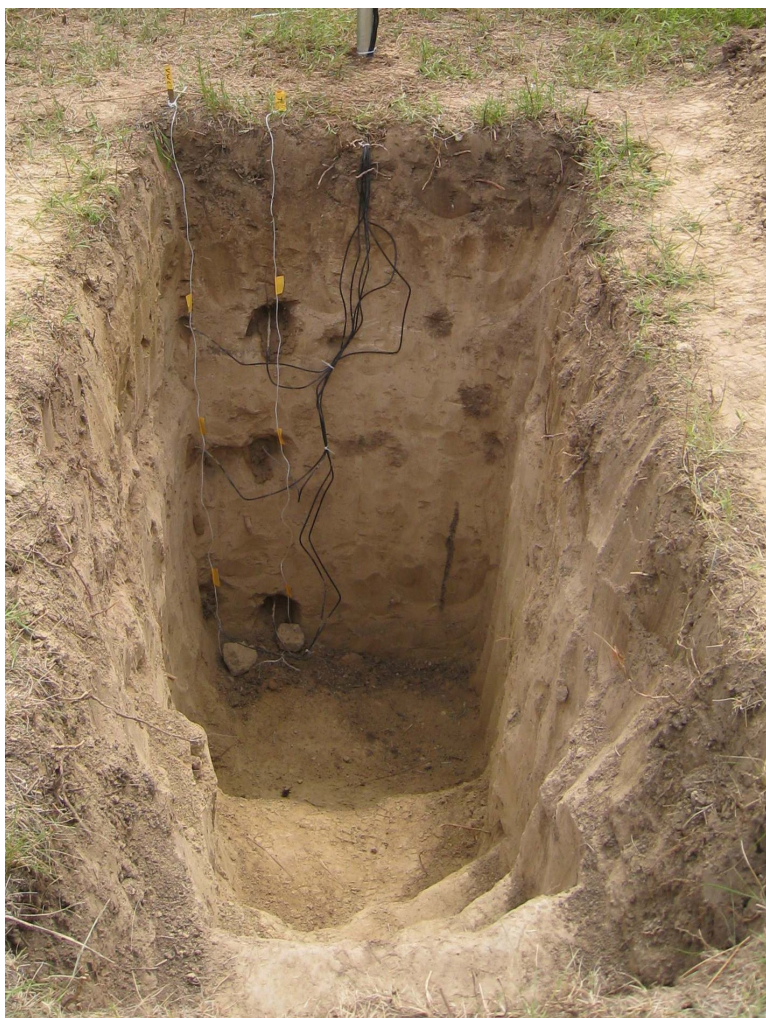
Fig. 2. An experimental site pit with three measuring points
