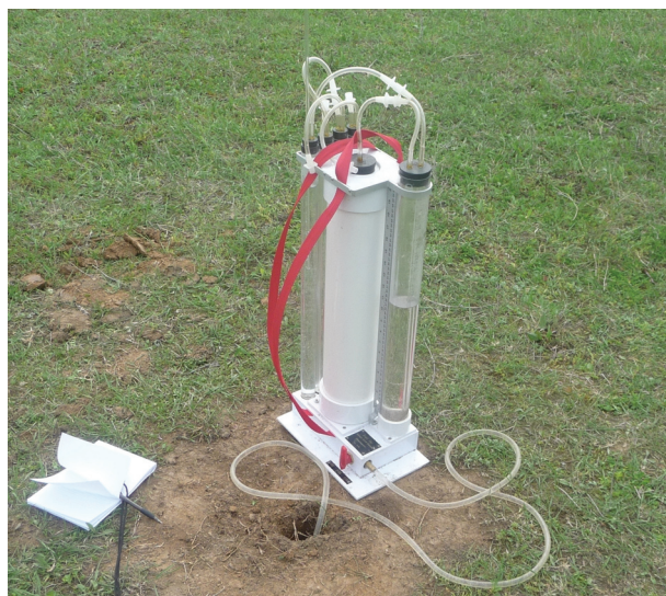
Fig. 1. A compact constant head permeameter test
