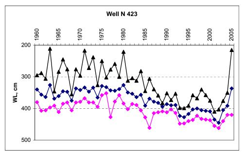
Figure 6. Annually maximal, average and minimal groundwater level for observational well N 423.
