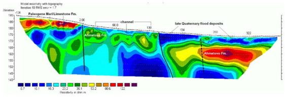
Figure 2. Interpreted 2-D-resistivity profile across Chirpan fault at Kopanite (V.E. = 2.5).
